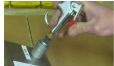
Step 4. Reduce the compressor output pressure (10 to 20 psi). Place one hand on the Outlet side of the valve while injecting air into the Inlet side of the valve. If you have cleared the debris – you will not feel any air coming out of the Outlet side of the valve. If you do feel air, repeat the steps above. If after repeated attempts you still cannot clear the debris, the AWEIS valve box must be replaced. **Normally the debris will clear after the first attempt.**
