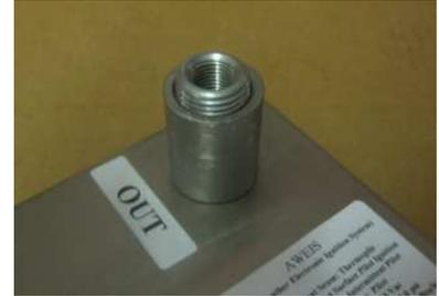
Step 2. Spray a small of lubricant in the Outlet side of the valve.
